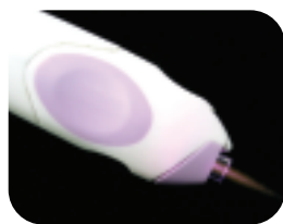
Plasma pulse from the Rhytec Portrait PSR 3 handpiece nozzle is characterized by a lilac glow transitioning to a yellowish light called a Lewis-Rayleigh Afterglow.
